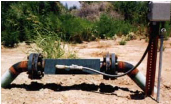
Figure 1: 4" Paraffin Control System installed on a 4.7-mile pipeline. Operator eliminated chemical cleaning, disposal, and maintenance, reducing paraffin to trace levels.
